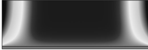
Fig. 5. Temperature distribution ( t = 600 s), T_{\min} = 288.15 K, T_{\max} = 288.32 K, scale: light color \rightarrow dark color means T_{\min} \rightarrow T_{\max}
